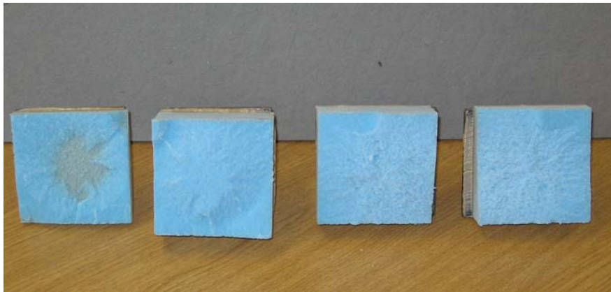
Picture showing the mode of failure
